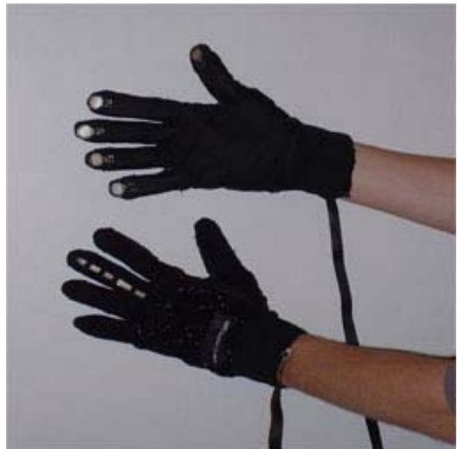
Below the visible part of the pressure-sensors, the homemade metallic sensors are sewed in. They consist of two different metallic wires that don't have any electrical contact with each other. When they strike a metallic surface a closed circuit is achieved.
